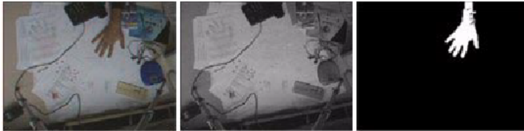
Image differencing with reference image. From left to right: input image, reference image, output image.
